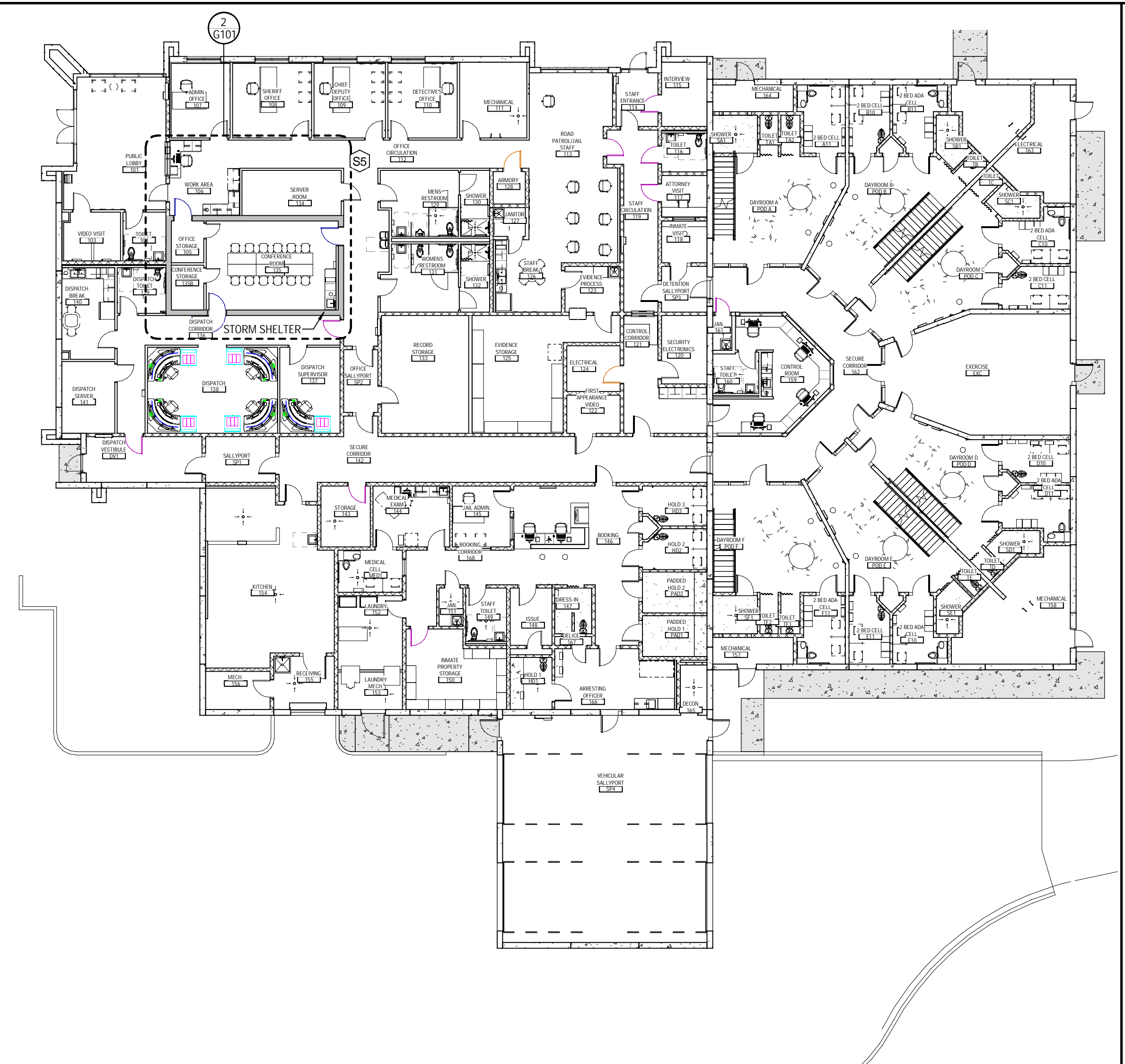
101 - FIRST FLOOR STORM SHELTER CODE PLAN 1/16" = 1'-0" (A2)/151
